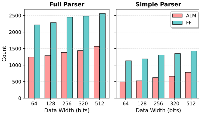
Fig. 6. ALM/FF utilization vs. datapath width for Altera Agilex 5 FPGAs.
